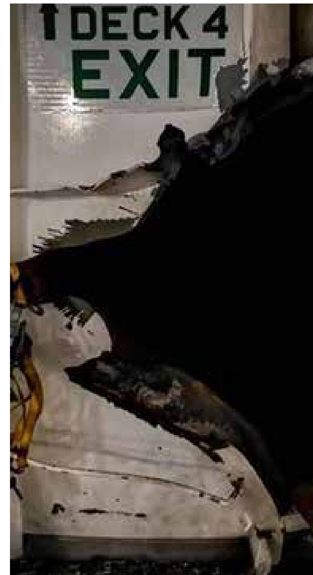
Hole in Israeli vessel Helios Ray caused by an Iranian limpet mine. (Ynetnews)
